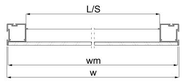
w = (W + 50 mm) : 3Door width Mirror width (glass) wm = w - 4 mmHorizontal profile Eden length - L L/S = w - 50 mmStrengthening profile length - S Spacer profile 04 length **S** + 46 mm
