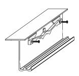
use self-tapping screw ∅3.5 or drill opening in track Ø 2.5 and use Unix screw Ø3.5
